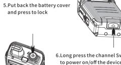
6.Long press the channel Switch to power on/off the device.
